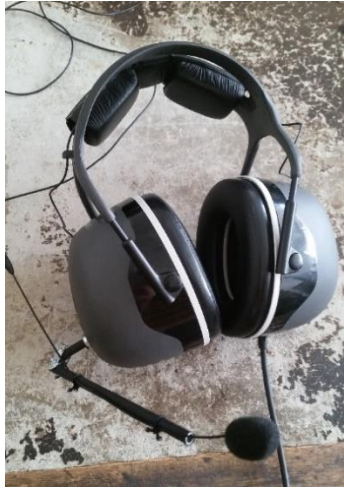
Figure 1. Specially built headphones with extra passive sound isolation.
